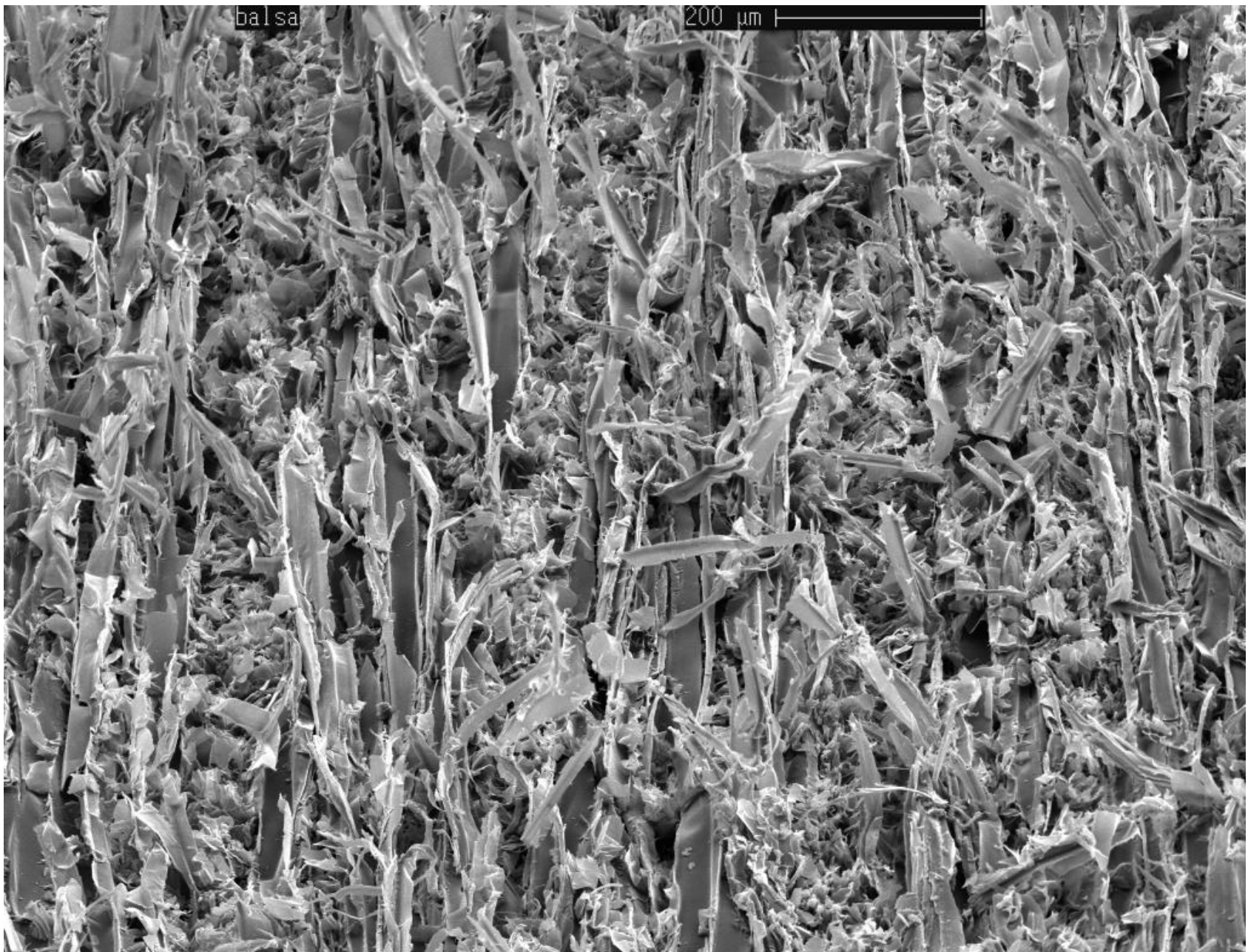
Balsa Sanded & Dry under the Electron Microscope
